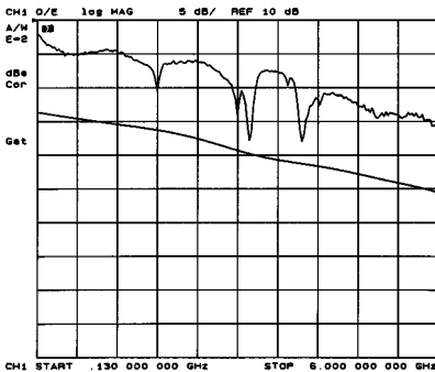
Figure 42. Frequency response with and without gating active (gated trace is offset)
